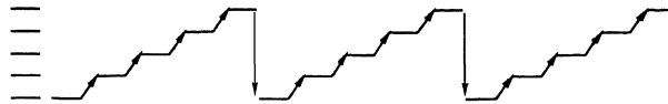
Fig. 4. Cascadic iteration: the problem is approximately solved on a coarser (lower) grid before interpolation to a finer (higher) grid is made. The cycle over all levels is repeated in an outer defect correction (iterative refinement) process. The levels used are the union of the grids \Omega_n , with |\mathbf{n}| = k, k = 1, 2, \dots, 10 . The number of points at each level is given in Table 1
