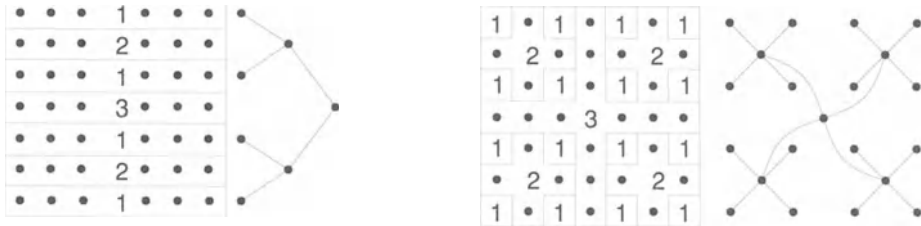
FIGURE 7. Stripe- and box-wise nested dissection decompositions and their parallelization structures.
