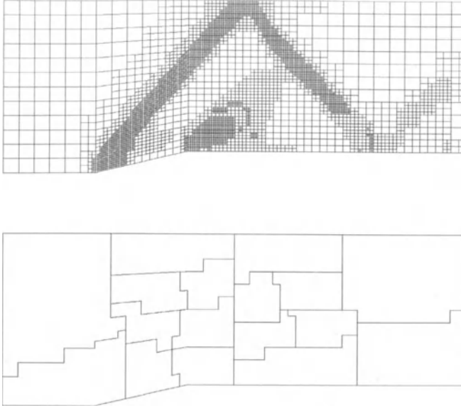
FIGURE 3. Mesh and partitioning at the 4th multigrid level
